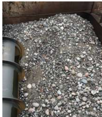
Figure 5.2-2 Rock dredged by hopper dredger, found inside the hopper
