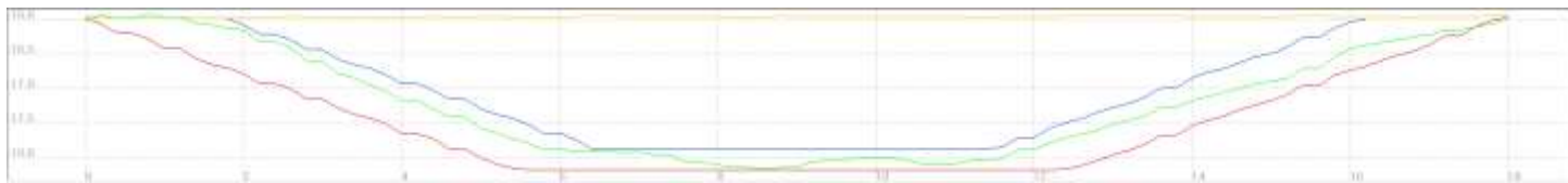
Figure 6-2 Achieved dredging accuracies. Blue and red line show tolerances. Green is the achieved result.
