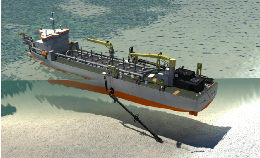
Figure 3-7: TSHD while removing rock from the seabed
