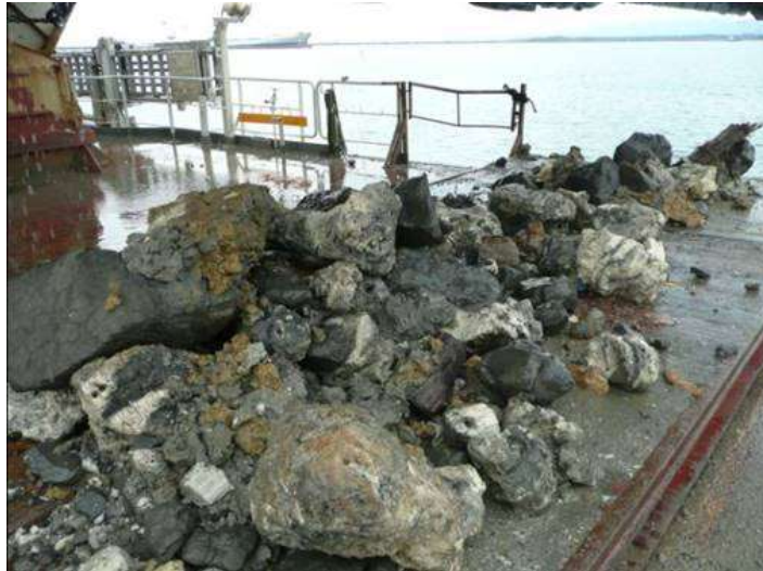
Figure 5.2-1 Rock dredged by hopper dredger, found under draghead
